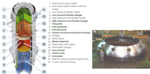
UK ABWR – the reactor
